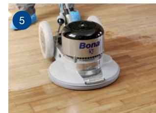
5 For oiled / hard wax oiled floors, buffer with Bona FlexiSand
